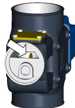
Figure 5. EGR valve. The arrow shows where the EGR damper is located
